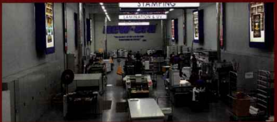
ABOVE: Bridge Publications' book printing plant in Los Angeles. The facilities include cutting, lamination, embossing, foil stamping, book case and binding stations. RIGHT AND BELOW: New Era Publications' facilities in Copenhagen, Denmark, a duplicate of the Bridge manufacturing plant in Los Angeles, but for production in 15 to 50 languages.
